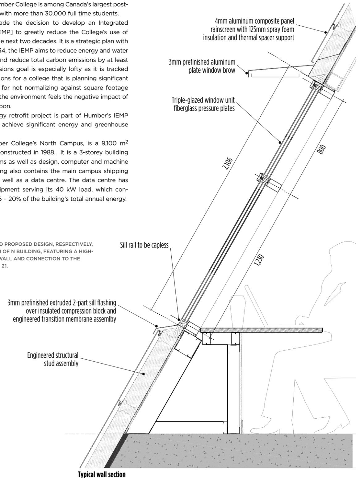
The exterior façade has sections of exposed structural concrete and masonry, sloped aluminum sandwich panels, and curtain wall glazing. Space conditioning is provided by a central chiller and steam boiler plant, which also serves much of the campus, as well as three roof top units [RTU's] with gas fired heating and direct expansion [DX] cooling. A dedicated cooling system provides chilled water for the data centre. Supply air is delivered to the spaces with variable air volume [VAV] systems.
